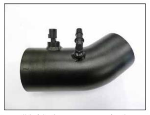
17. Install the inlet air temperature sensor into the AIRAID® intake tube as shown.
