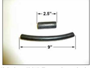
19. Cut the provided ½" silicone vent hose to a length of 9" long, and cut the 5/8" vent line to a length of 2.5" long.
