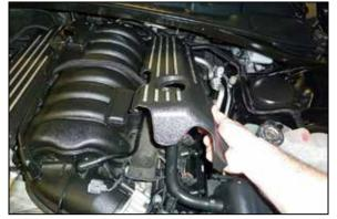
3. Lift up and remove the driver side ignition coil cover
