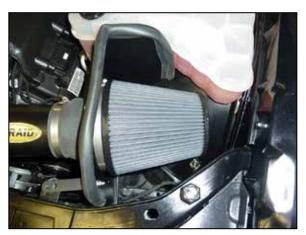
24. Install the AIRAID® air filter and secure with the provided hose clamp.
