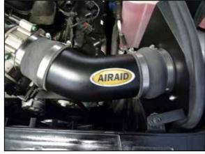
18. Install the AIRAID® intake tube into the silicone hump hose and then into the into the silicone step hose at the throttle body. Align the intake tube and heat shield for proper fit and then secure the intake tube with the provided hose clamps and the heat shield bracket with the factory air box retaining bolt removed in an earlier step.
