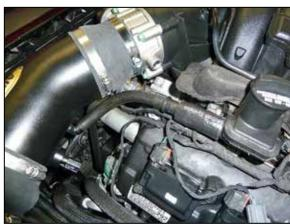
21. Install the assembled vent hose onto the fitting installed in the AIRAID® intake tube and then attach the open end to the valve cover port.
