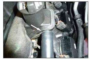
4. Disconnect the crank case vent hose from the valve
