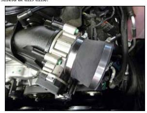
14. Install the step hose (08497) onto the throttle body and secure with the provided hose clamp.
